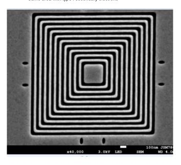
photomicrographs. Please note the contrast depends upon illumination and is not particularly high. For instruments with verniers or electronic calipers distance measurements can be verified using a pitch pattern of appropriate size. The standard is ideal for measuring modulation transfer functions.
