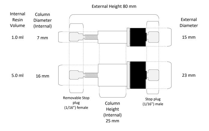
NOTE: HiFliQ FPLC columns are supplied with a moulded removable (1/16") female stop plug attached to the (1/16") male outlet port. Remove prior to use, reverse and use to seal the column for storage.
