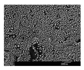
the 'standard' Agar gold on carbon specimen, AGS168. Many of the instructions given on the AGS168 technical leaflet apply also to these ultra-high resolution test specimens, but it should be noted that the instrumental magnification required to resolve the smaller particles, will be higher.
