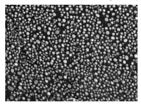
These gold on carbon calibration specimens have been specifically produced to enable the ultra high resolution capabilities of the current generation of high performance scanning electron microscopes to be assessed. In particular, the AGS1969 sample with its ultra small gold particle size (<3nm-50nm) is designed for use with SEM's equipped with field emission guns.
