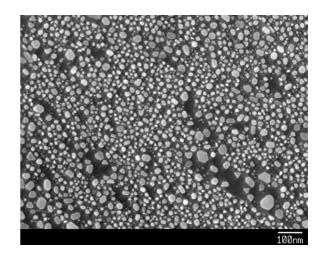
gold on carbon specimen, AGS168. Many of the instructions given on the AGS168 technical leaflet apply also to these ultra-high resolution test specimens, but it should be noted that the instrumental magnification required to resolve the smaller particles, will be higher.
