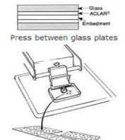
Fresh material is cut on a Vibratome®, treated with HRP and placed on ACLAR cut into a slide shape - observe under LM - if OK, process for TEM on the slide.
