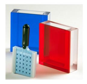
The 22510 Grid Staining Matrix System consists of four components: The Staining Matrix Body with handle; Matrix cover and two Staining Vessels.
