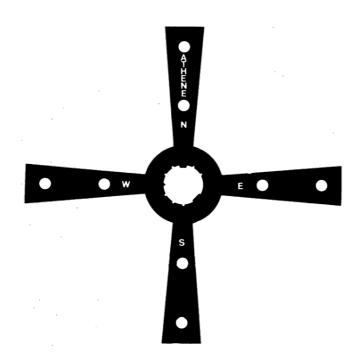
This consists of an inner ring of 4mm diameter (outside) and 2mm inside diameter. It has four arms each extending 6mm outwards.
