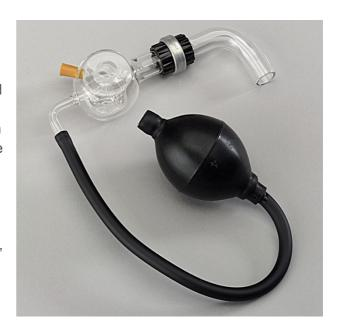
All the sprays will operate with a very small quantity of liquid suspension. The Mk II version now available will operate with only 0.1 to 0.2 ml of liquid and is therefore particularly suitable for concentrated virus preparations. It will yield droplets down to 1um in diameter.
