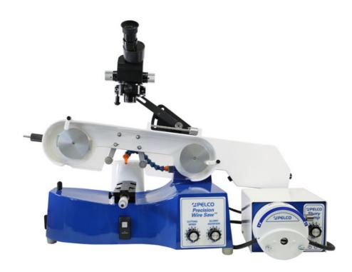
The PELCO® Precision Wire Saw™ is capable of cutting a variety of materials while minimizing damage from the cutting process using a gentle lapping action. This gentle action combined with high precision and low kerf damage makes the Diamond Wire Saw ideal for slicing samples where minimizing mechanical damage and precise positioning of the cut are critical. This wire saw is an updated version of the South Bay Technology Model 850 Abrasive Slurry Saw / Wire Saw.
