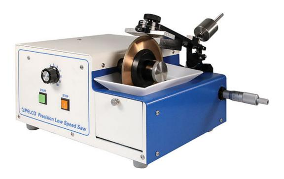
The PELCO® Precision Low Speed Saw is a compact, multipurpose, precision saw designed to cut a wide variety of materials with minimal subsurface damage. Its low speed makes it possible to cut fragile materials that would otherwise fracture as well as soft materials that would load the diamond wheel on a higher speed saw. A variety of sample holders are available, providing a means for mounting any shape of sample, while multi-axis goniometer adaptability simplifies cutting oriented crystals.
